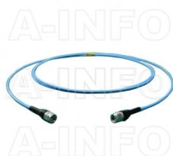
1.85M-1.85M-B010-2000 Flexible Cable Assembly 2000mm DC- 67GHz 1.85mm Male to 1.85mm Male
